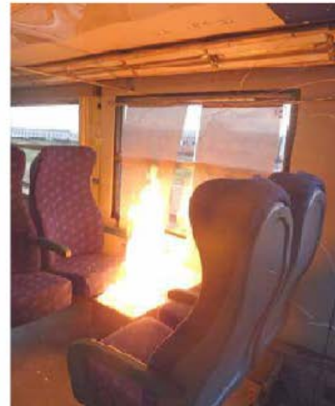
The first FTIR picks the gases directly on the fire vertical.
